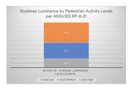
in the chart at left, we see an example of the required luminance level for a Local road with an R<sub>2</sub> or R<sub>3</sub> surface (asphalt surfaces commonly used in North America for local roads).
